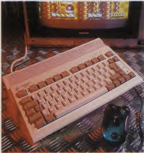
Most factory fresh A600s and A1200s have swarfy disk drives – use a vacuum cleaner to suck the rubbish out!
